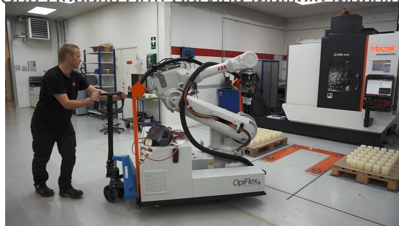
One Robotic Arm Serving Multiple Machines
