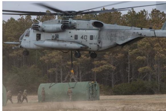
Marines deploy a section of a floating bridge system during a field exercise at Camp Lejeune
